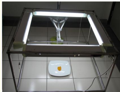
**Figure 1:** The experimental setup of the lighting system, digital camera, and food sample.
